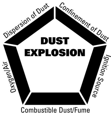
**FIGURE 3** – The management or removal of one or more of the elements in the Explosion Pentagon can reduce the explosion risk.
