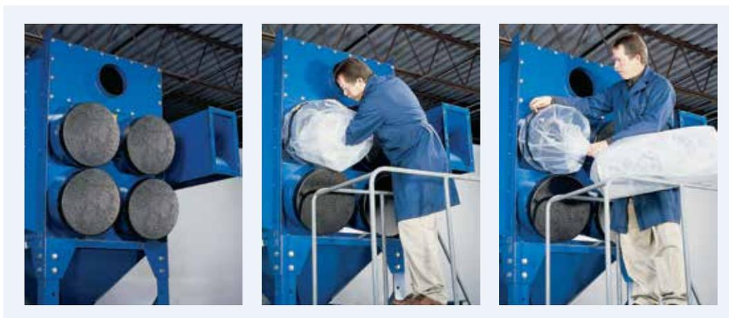
**FIGURE 4** – The Bag-In/Bag-Out (BIBO) improves filter changeouts and hopper discharge maintenance to help minimize worker exposure to potentially harmful dusts and reduce exposure of contaminants to the atmosphere.
