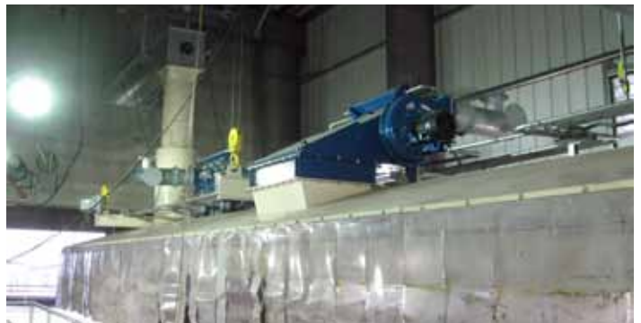
Dust collectors with fluted filter packs are much smaller than conventional dust collectors, which allows the collector to be integrated into a truck load-out hood.
